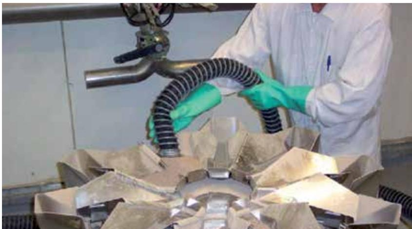
*Figure 9: Vacuum cleaning granules from partially dismantled packaging equipment using a special industrial vacuum cleaner with HEPA filter to control dust.*
