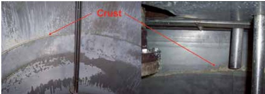
*Figure 4: Visual inspection of the interior of a reactor revealing unwanted material is still present, and therefore, further cleaning is required.*
