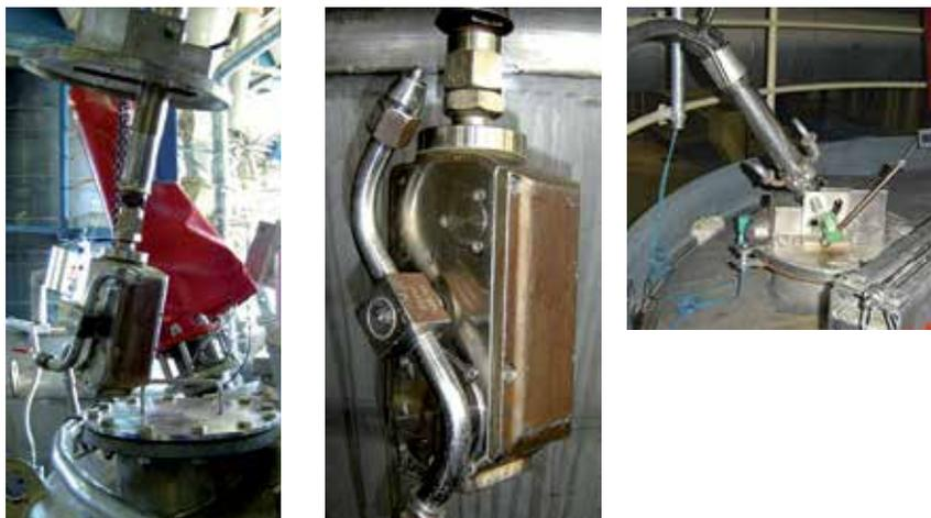
*Figure 6: Mobile spray head for reactor and tank cleaning. To be installed on a free flange and connected to a high pressure water supply. The spray head is rotating vertically and horizontally around the pipe axis.*
