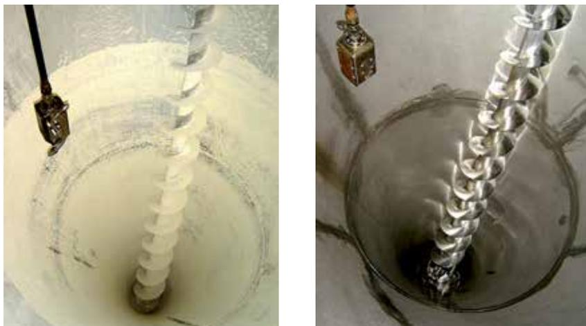
*Figure 5: Interior of a mixer before and after wet cleaning using a rotating spray head, followed by drying*
