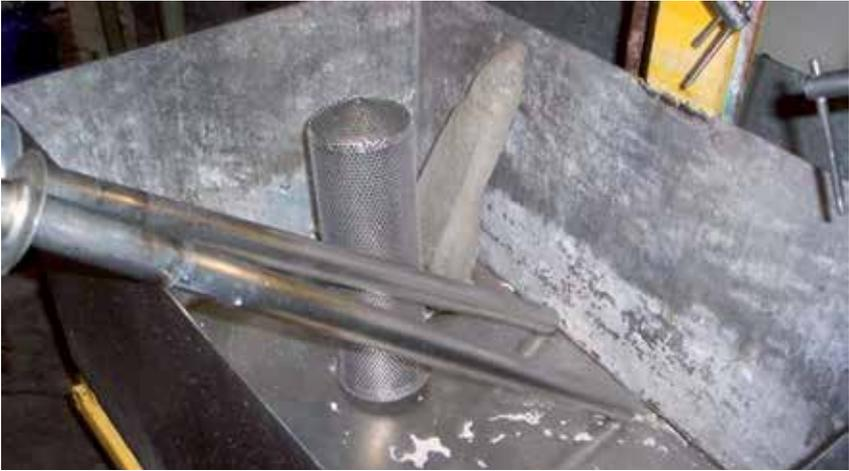
*Figure 7: Workstation for the mechanical, manual cleaning (“brushing”) of small, dismantled equipment parts.*
